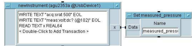
Fig. 3: SCPI commands written in Direct IO object to obtain measurements from DAQ card
